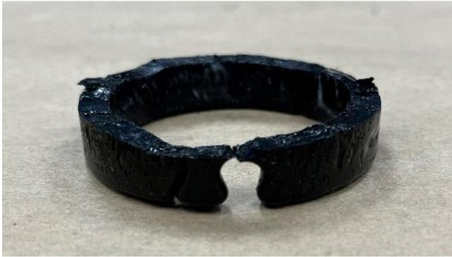
**Figure 50: Poorly Molded Aged Roofing Binder Specimen for ABCD Test**
