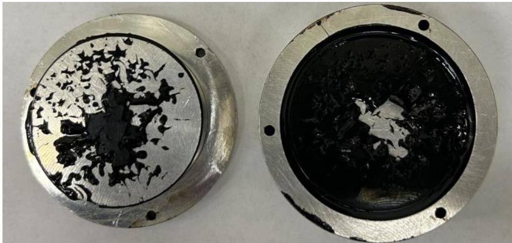
**Figure 48: Poker Chip Test for Material M1-S (71) at 30°C, Showing Issues with Debonding during the Procedure**
