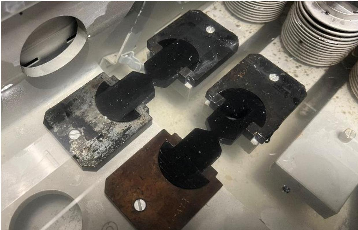
**Figure 15: Molded SDENT Specimens (5-mm Ligament Length)**
