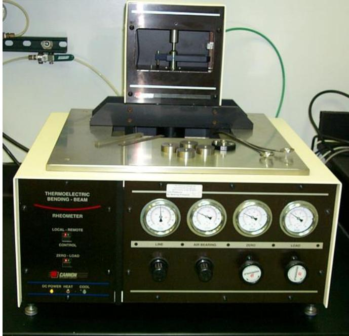
**Figure 7: Bending Beam Rheometer (BBR) Test Equipment**
