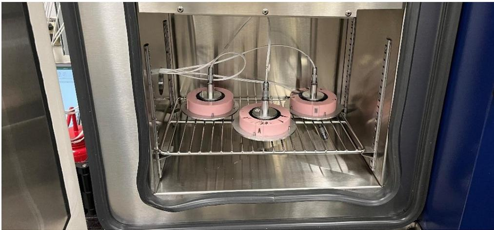
Figure 13: ABCD Specimens in Environmental Chamber
